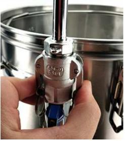
We must stress not to rotate the rotating racking arm while it is engaged in the lock down position. If you need to rotate the racking arm to fill your fermenter, please switch off the pump and readjust the camlock to the position you need then reengage the camlock.
