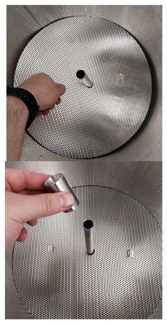
Once you have fitted the top screen use the stainless siphon cone and place this over the extension tube with the cone side facing up. Push down on the cone until the extension tube and cone is sitting gently against the top screen. (shown to the left)
